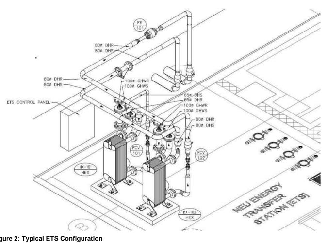
Figure 2: Typical ETS Configuration
