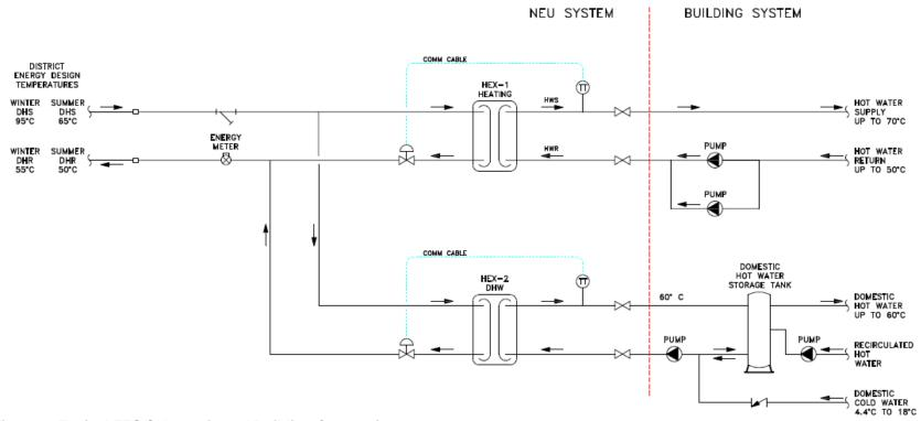
Figure 3: Typical ETS Schematic and Building Connection
