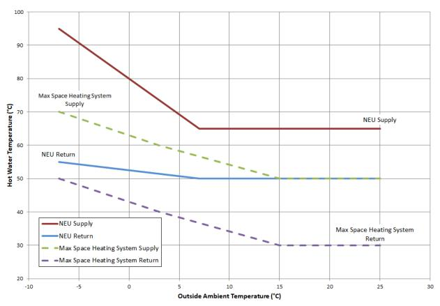
Figure 4: NEU System and Building Heating System Temperatures
